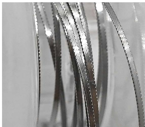
شکل ۲ 010 × 029 inch Stainless steel multi strand Flattened wire
