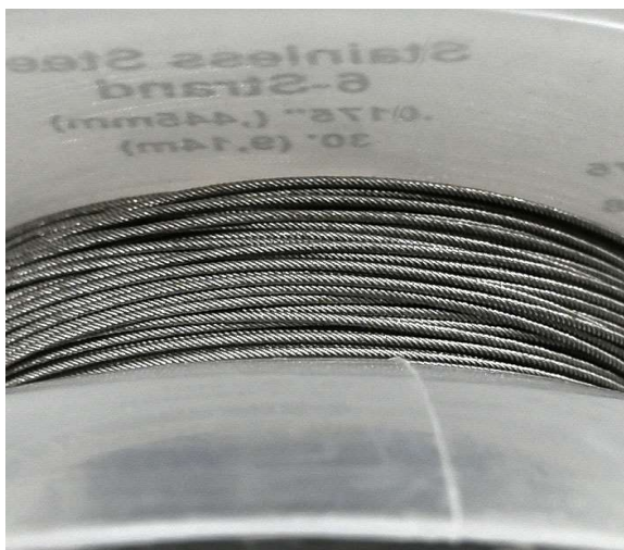
شکل ۳- 0/0175 stainless steel 6 –strand Coaxial wire
